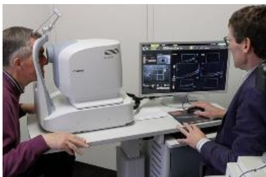
An Optical Coherence Tomography scanner
